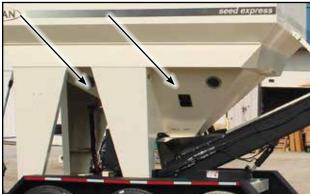
Fig 39 - Sample slide gates
