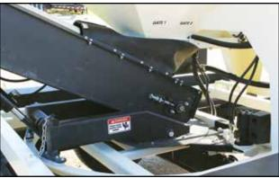
Fig 41 - Conveyor hopper on turntable platform
