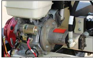
Fig 54 - Engine and hydraulic pump
