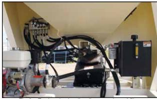
Fig 8 - Engine, hydraulic oil reservoir and filter
