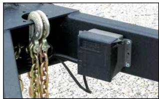
Fig 16 - Break-Away system control box
