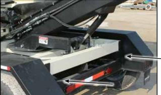
Fig 67 - Weigh scale load cell location
