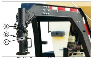
Fig 31 - Gooseneck hitch components
