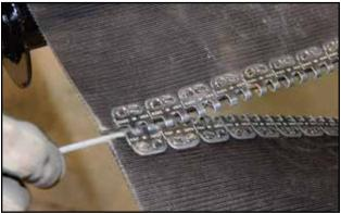
Fig 58 - Thread lacing cable
