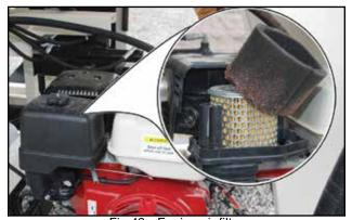
Fig 49 - Engine air filter
