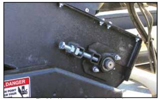
Fig 56 - Hopper roller tension bolt
