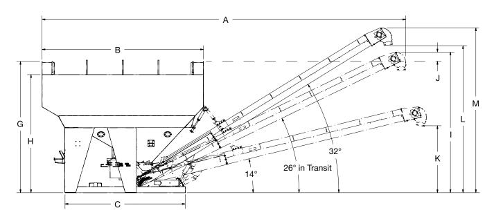
Fig 70 - Measurements of 375 RT tender
