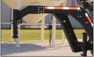
Fig 29 - Gooseneck hitch
