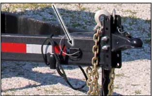
Fig 17 - Break-Away cable on hitch tongue
