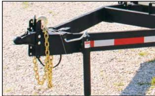
Fig 15 - Tongue on a bumper hitch trailer
