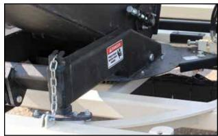
Fig 42 - Turntable platform anti-rotation chain
