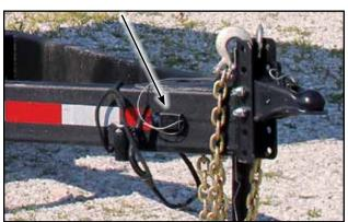
Fig 64 - Break-Away cable on hitch tongue
