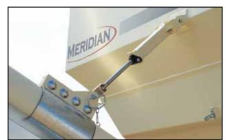
Fig 26 - Conveyor tube transport lock w/ damper mechanism
