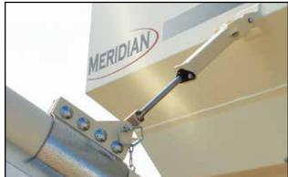
Fig 43 - Conveyor tube transport lock and damper mechanism
