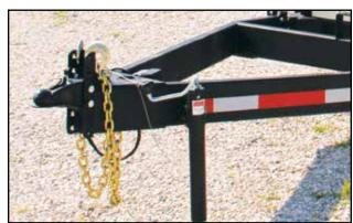
Fig 27 - Trailer hitch with safety chains
