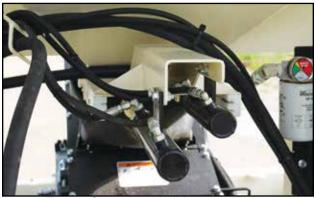
Fig 11 - Compartment slide gate cylinders
