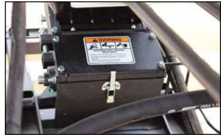
Fig 48 - Conveyor tube access door
