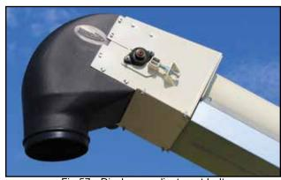
Fig 57 - Discharge adjustment bolt
