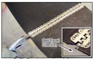
Fig 60 - Crimp lacing and taper belt corner
