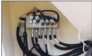
Fig 53 - Hydraulic valve manifold
