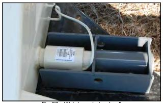
Fig 68 - Weigh scale load cell
