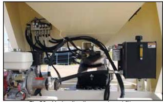
Fig 52 - Hydraulic oil reservoir and filter
