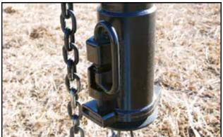
Fig 32 - Gooseneck trailer coupler
