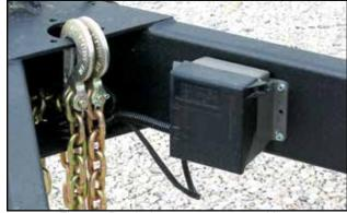
Fig 63 - Break-Away system control box
