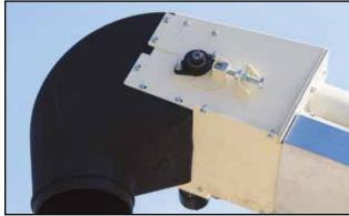
Fig 51 - Discharge roller bearing
