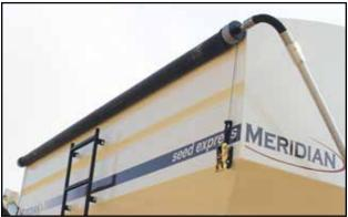
Fig 13 - Roll tarp and crank handle
