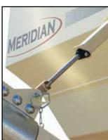
Fig 47 - Secure conveyor tube for transport
