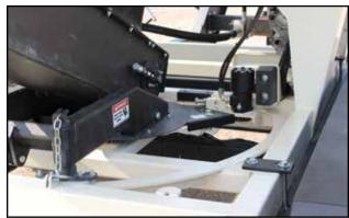
Fig 9 - Conveyor tube rotating system
