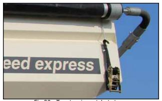
Fig 36 - Tarp tension ratchet straps
