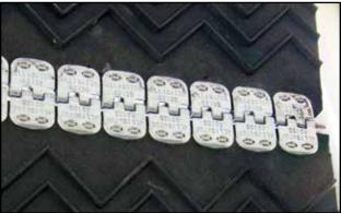
Fig 59 - Conveyor belt lacing
