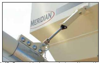
Fig 10 - Conveyor tube damper mechanism and transport lock
